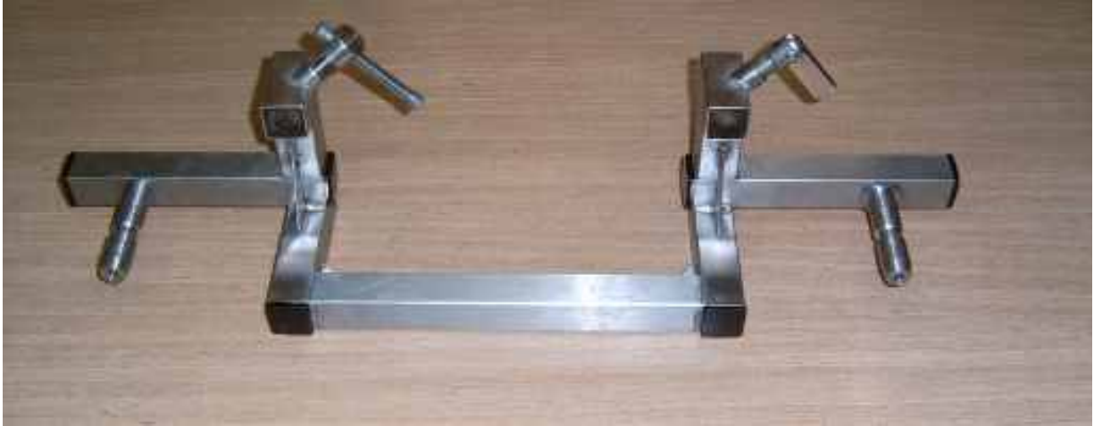
MODIFICATION FOR OPERATING TABLE HEAD END
